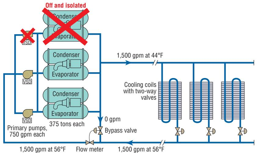
**FIGURE 6.** At 50-percent load, one pump and one chiller in this VPF arrangement have cycled off, and the chiller has been isolated from any water flow. The water-flow rate is well above the minimum of 250 gpm, so the bypass pipe is not used.
