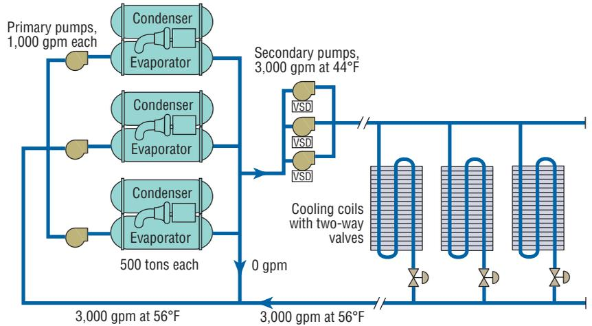
**FIGURE 2.** The flow of chilled water in the primary loop of a P/S system is constant, while two-way valves and variable-speed-driven pumps in the secondary loop control coil capacity by varying water flow. Ideally, delta-T in the coils remains constant.
