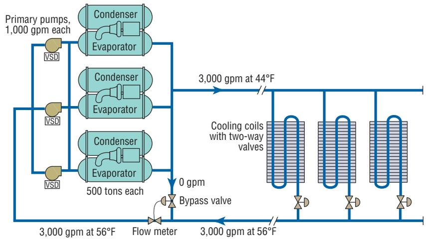
**FIGURE 5.** Like a P/S configuration, a VPF configuration uses two-way valves and variable-speed-driven pumps to vary water flow and control coil capacity, while delta-T remains relatively constant. However, there is only one water loop, and water flow is varied throughout the chilled-water circuit.
