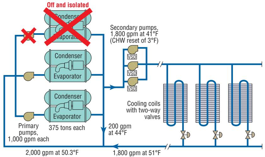
**FIGURE 8.** This P/S system, operating at 50-percent load and 8°F delta-T, requires 2,250-gpm coil flow and operation of three chillers. Resetting the supply temperature by 3°F to 41°F results in 10°F delta-T, coil flow of 1,800 gpm, and the need to operate only two chillers.
