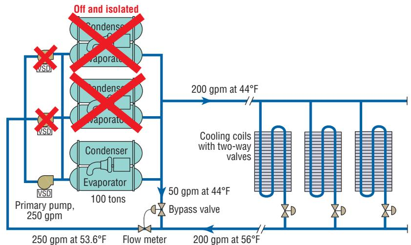
**FIGURE 7.** At 33-percent load, a second chiller and chilled-water pump cycle off. When the flow meter senses that flow in the main circuit has fallen to the 250-gpm minimum, it begins to open the bypass valve. At 6.7-percent system load, flow through the coils, bypass pipe, and evaporator is 200 gpm, 50 gpm, and 250 gpm, respectively.
