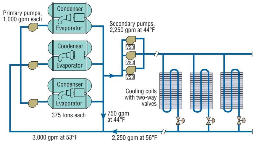
**FIGURE 3.** At 75-percent load, the flow of chilled water in the primary loop of a P/S system is constant at 3,000 gpm, while two-way valves and variable-speed-driven pumps throttle water flow through the coils to 2,250 gpm, approximately 75 percent of design value. The 750 gpm of excess water from the primary loop flows through the decoupler pipe.
