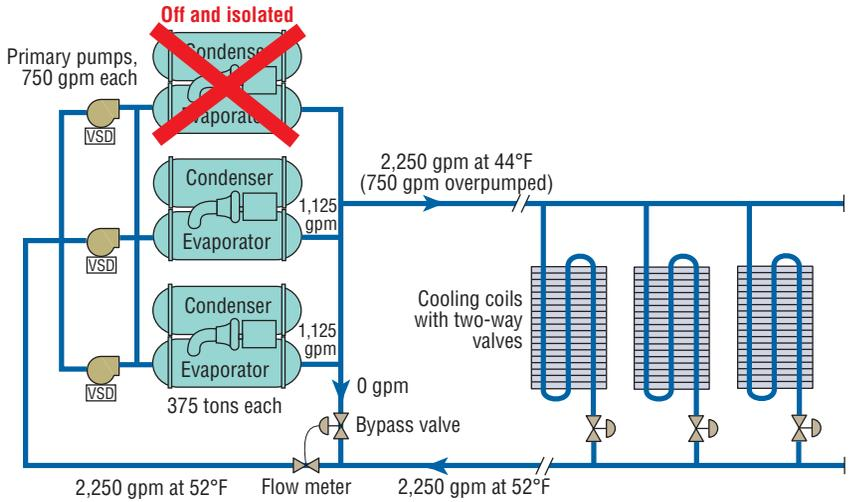
**FIGURE 9.** In this 50-percent-loaded VPF system with low delta-T of 8°F, two chiller systems cannot cool the 2,250 gpm needed to meet the load. If the third headered pump is activated and the two active chillers are overpumped, however, the load can be met.
