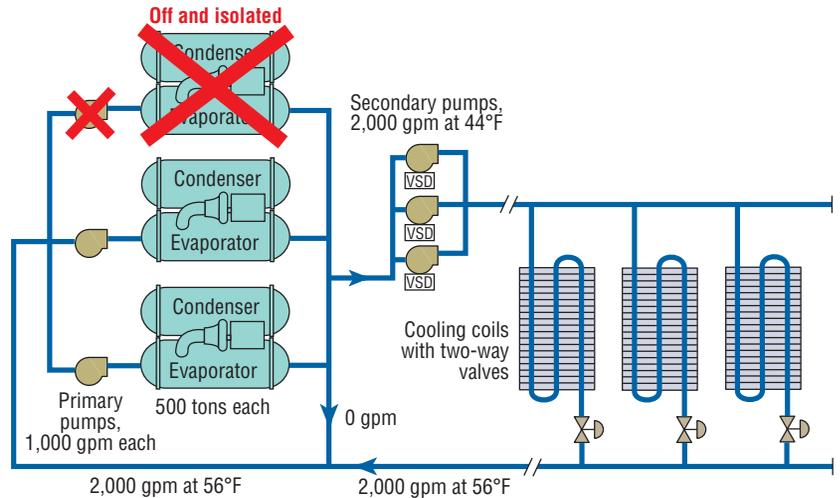
**FIGURE 4.** Below 67-percent load in a P/S system, one of the chillers and its chilled-water pump can be cycled off. Water flows adjust to rebalance the system.
